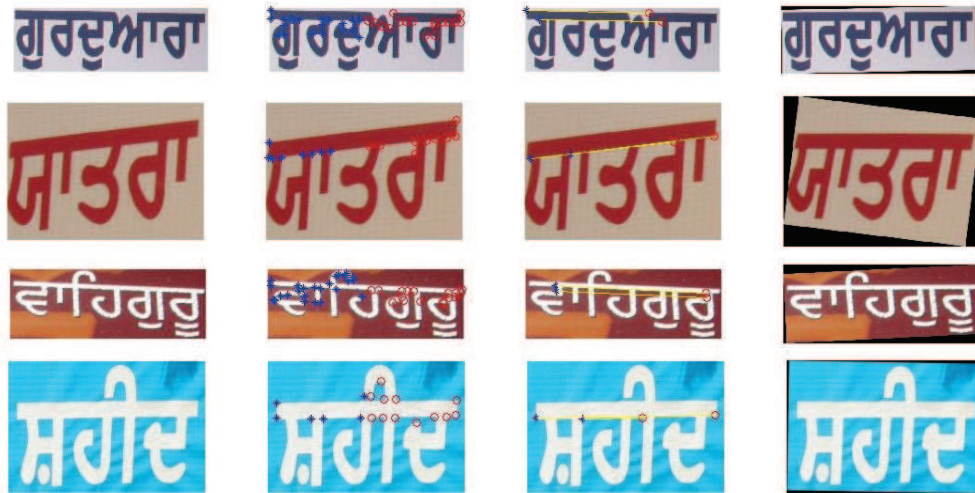
FIGURE 3. Skew correction of Gurmukhi words, from left to right: Original image, Salient points, Identified parallel lines and skew corrected image
