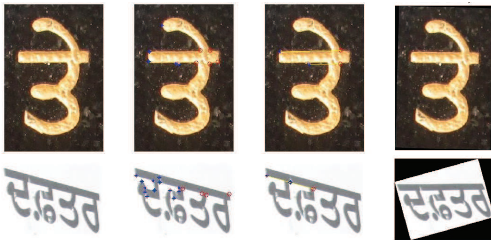
FIGURE 4. skew correction of single character and severely skewed words
