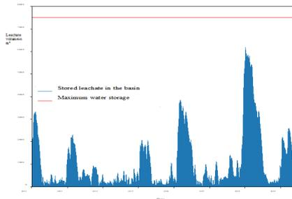
FIGURE 1. The recent leachate and whole capacity in the pool sink for 2704 days
